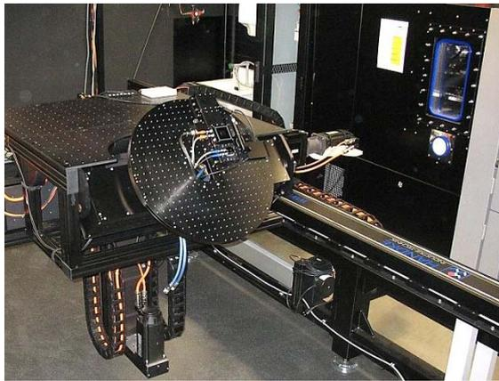
Fig. 1: On the left-hand side, the integrated solar cell goniometer can be seen. The quartz glass entrance window of the climate chamber is located in the top right corner of the image. A mirror (not shown here) on the xyz-table will reflect the monochromatic and the bias beam to a solar cell inside the climate chamber [1].
