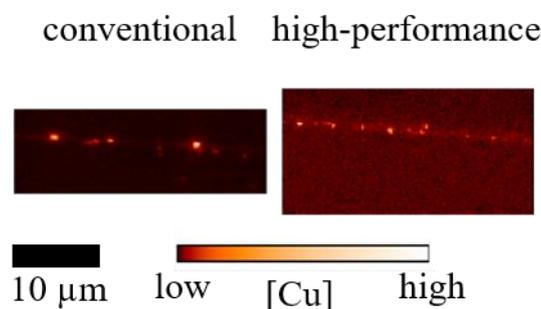
Figure 1: Synchrotron  $\mu$ -XRF maps of copper concentration at grain boundaries with 18.6° and 18.3° misorientation in conventional and high-performance multicrystalline silicon, respectively. Maps are 30  $\mu$ m wide, with 200 nm full-width at half-maximum beam diameter and 220 nm pixel size.
