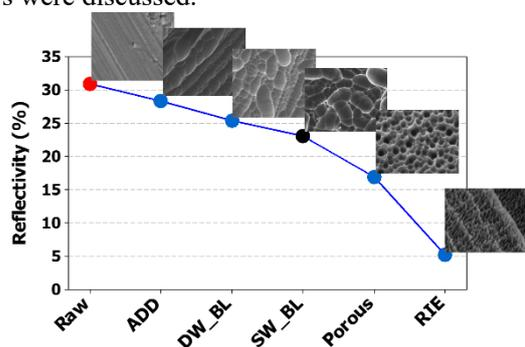
Fig.1 Reflectivity of raw and textured DW mc-silicon wafers
