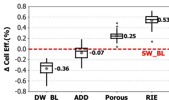
Fig.2 Cell performance of several textured DW mc-silicon wafers
