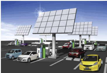
Figure 1: Illustration of the EV solar station that absorbs surplus energy from the PV on the car-roof.
