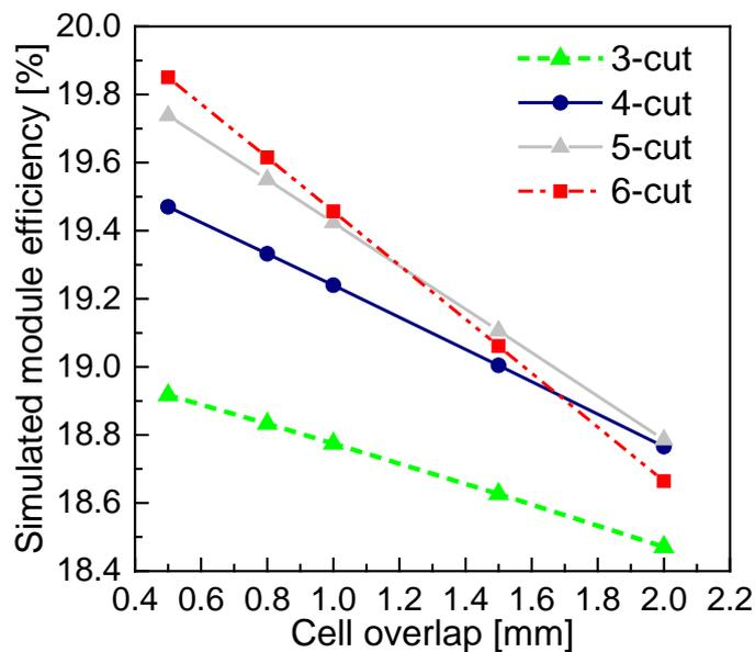
Figure 1: Simulated efficiency of shingled bifacial PV module for varying cell overlap and number of cell cuts.
