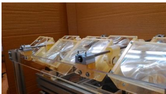
Figure 1: Photograph of a prototype 2-axis microtracking system for CPV
