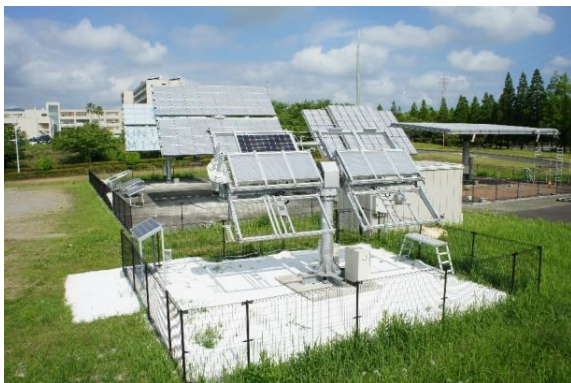
Figure 1: Photograph of 3 months after the white foam glass spread.
