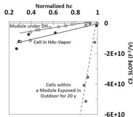
Figure 3: Correlation of  $I_{sc}$ -reduction and  $C_3\_SLOPE$ .
