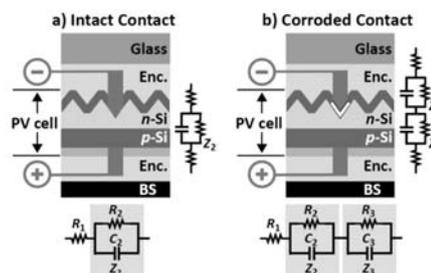
Figure 1: Evolution of AC equivalent circuit by corrosion.
