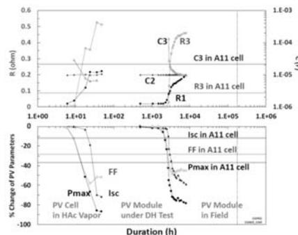
Figure 2: Evolution of AC impedance and  $I$ - $V$  characteristics during two acceleration tests and those in fielded PV module.
