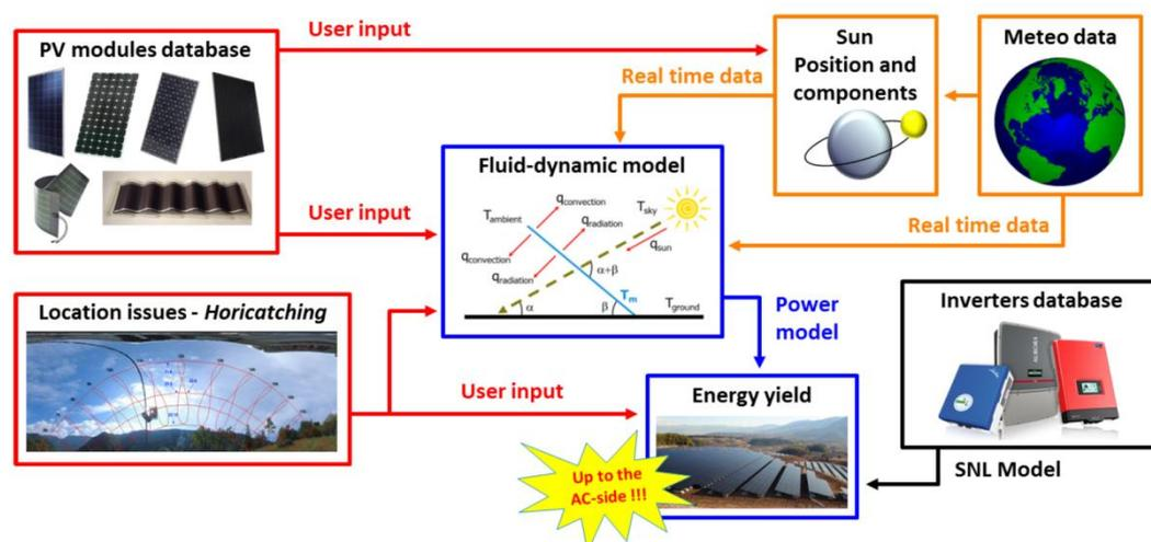
Figure 1: Schematic of our modelling platform. From the estimation of the PV module irradiance and temperature, the choice of the inverter, the time-dependent power model predicts the instantaneous power produced by the EIPV system at the AC side.
