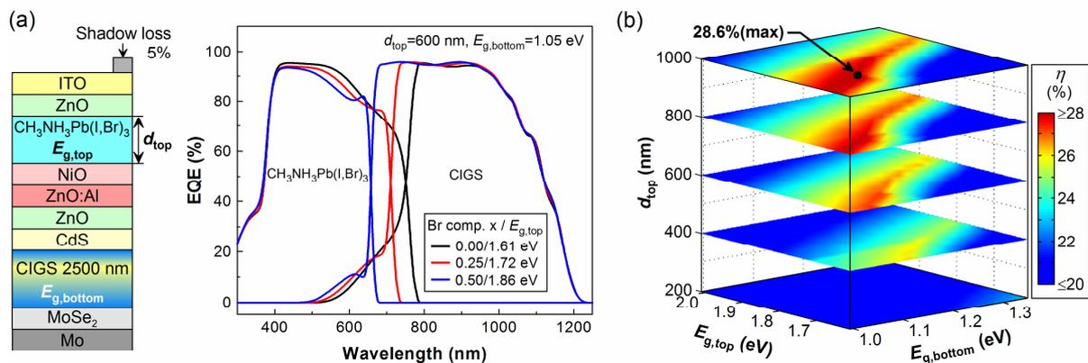
Figure 1: (a) Assumed device structure and the EQE simulation results and (b) conversion efficiencies of the tandem solar cells as functions of  $E_{g,\text{top}}$ ,  $E_{g,\text{bottom}}$  and  $d_{\text{top}}$ .
