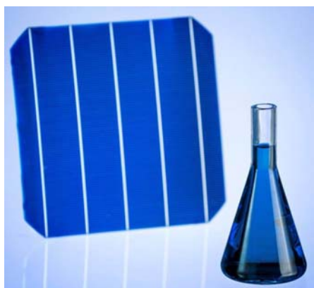
Figure 1: 20.2% efficient BackPEDOT solar cell fabricated on a large-area Cz-Si wafer ( 15.6 \times 15.6 \text{ cm}^2 ) with a 5-busbar screen-printed front Ag grid. The container is filled with the non-toxic aqueous dispersion of PEDOT:PSS (~98% water), which is suitable for deposition methods based on aqueous solutions such as spin-coating, spray-coating or slot-die-coating.
